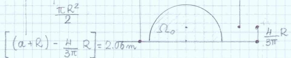
$$(\downarrow) F_{az} = \gamma V_{\square} = \gamma \left[ \frac{\pi R^2}{2} (a+R) - \frac{\pi R^3}{3} \right] = 18.4 \text{ kN}$$
