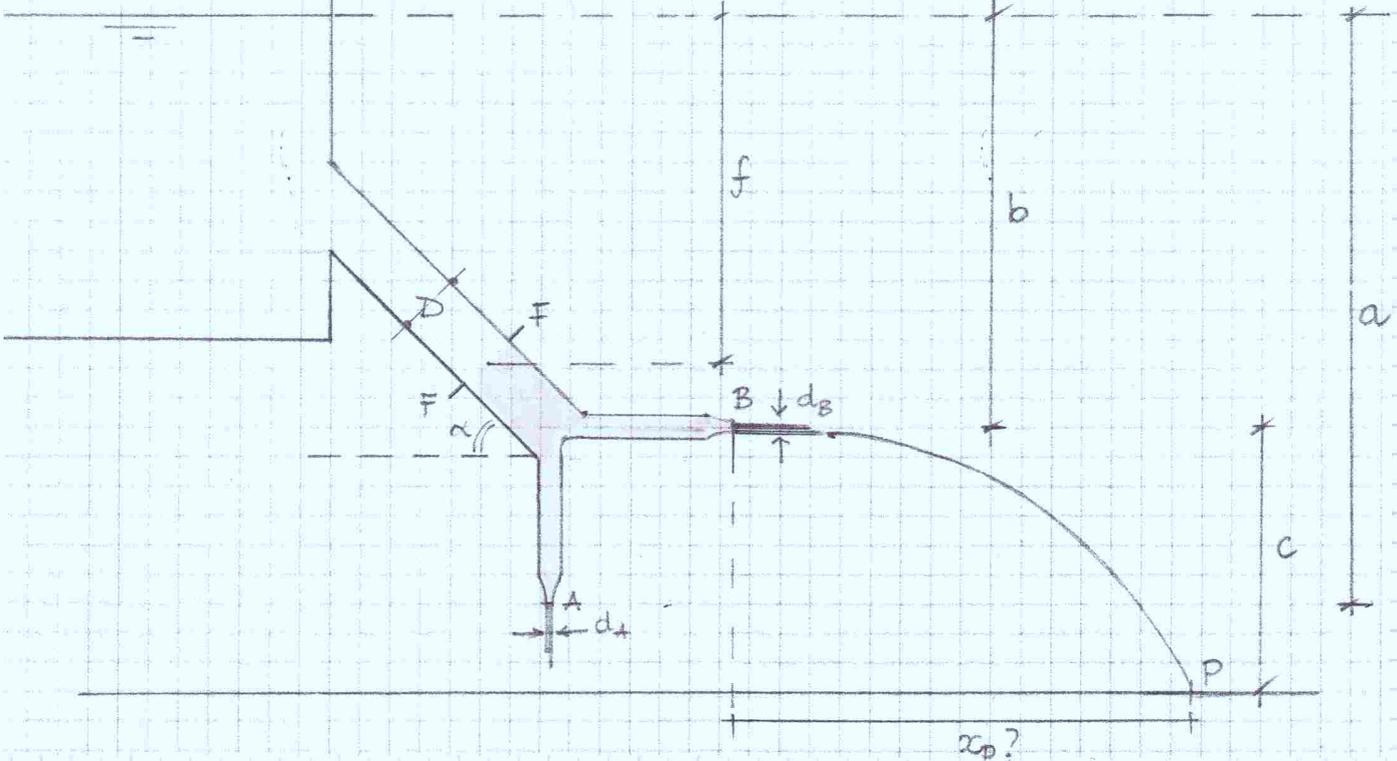
$$v_B = \sqrt{2gb} = 7.00 \frac{m}{s}; Q_B = v_B \omega_B = 35.2 \frac{l}{s} \quad v_A = \sqrt{2ga} = 7.67 \frac{m}{s}; Q_A = 21.7 \frac{l}{s}$$
