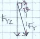
$$F_r = \sqrt{F_{rx}^2 + F_{rz}^2} = 327 \text{ N} \quad \theta = \arctg \left| \frac{F_{rz}}{F_{rx}} \right| = 74.4^\circ$$
