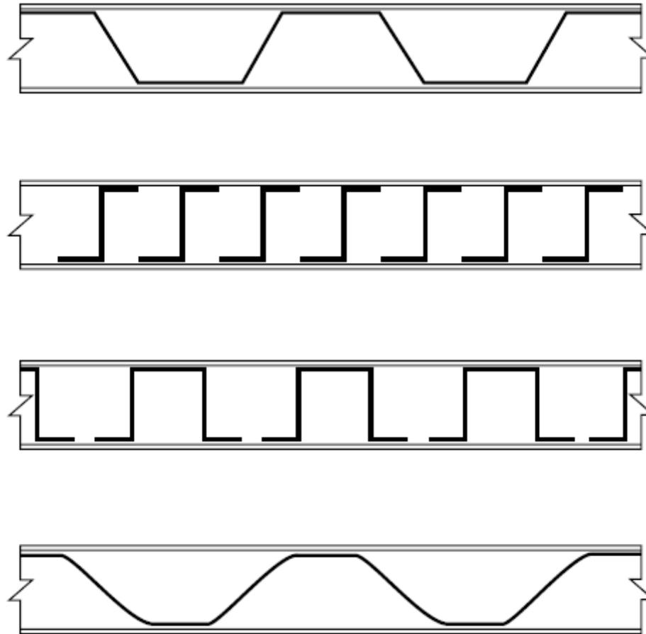
Figure 10.2.4 Steel sandwich plates with various core shapes.
