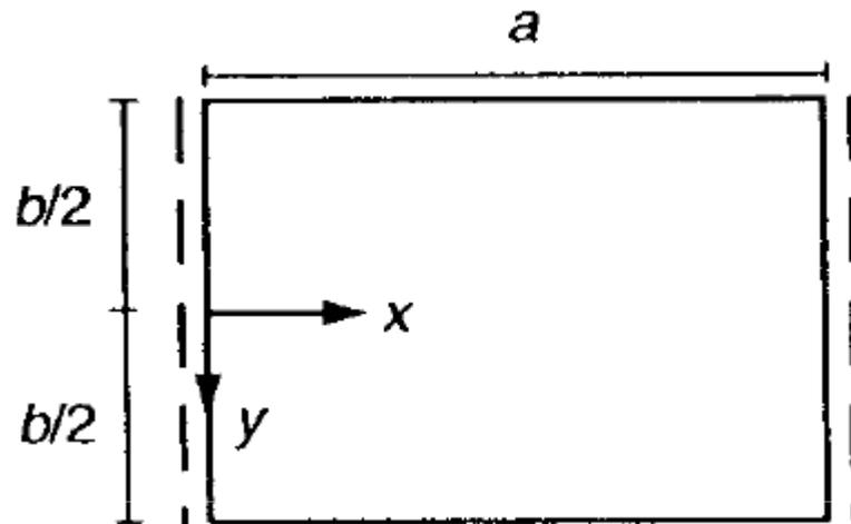
$$w = 0 \quad \frac{\partial^2 w}{\partial x^2} = 0 \quad \text{in} \quad x = 0, a$$
